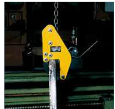
TWG with modified side plates for use in confined spaces (e.g. lathe machine).
