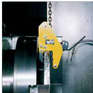
TWG with modified side plates for use in confined spaces (e.g. lathe machine).
