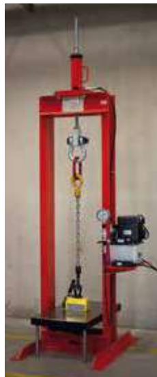
Permanent load lifting magnet TPM 0,3 for a test in the test rig RPYS-1215 complete with the test plate AYP-1215-S
